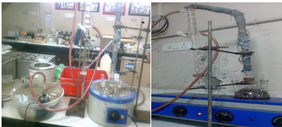
Figure 2: Hydro-distillation using Clevenger Apparatus
